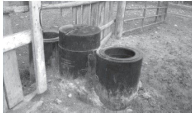
Kornfeld Ranch, Val Marie, SK (306-298-4629) Thermosink Energy-Free water trough using pressurized waterline.
